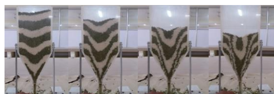
t=1 sec (a) t=3 sec (b) t=5 sec (c) t=7 sec (d) Thickness of rice layer = 2 cm Thickness of Moong Dal=3.5 cm Angle of repose = 60°
