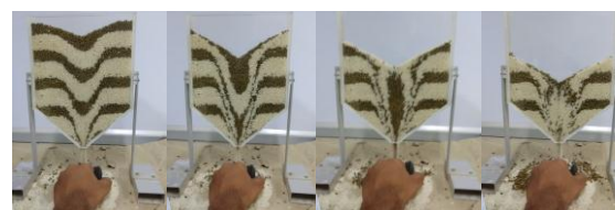
t=1 sec (a) t=3 sec (b) t=5 sec (c) t=7 sec (d) Thickness of rice layer = 3.5 cm Thickness of Moong Dal=2 cm Angle of repose = 45°
