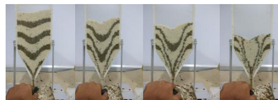
t=1 sec (a) t=3 sec (b) t=5 sec (c) t=7 sec (d) Thickness of rice layer = 3.5 cm Thickness of Moong Dal=2 cm Angle of repose = 60°
