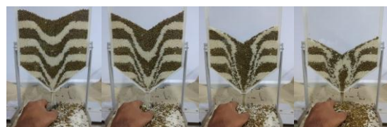
t=1 sec (a) t=3 sec (b) t=5 sec (c) t=7 sec (d) Thickness of rice layer = 2 cm Thickness of Moong Dal=3.5 cm Angle of repose = 45°
